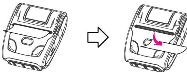
5. To change paper width, move paper guide while pressing paper width change button as shown in the picture.
