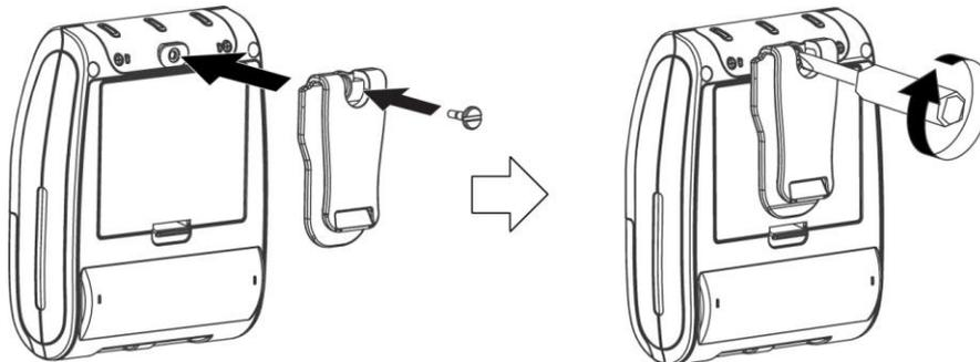
Following the instruction of the arrow, please put the belt clip in the hole and turn and fix the screw to the right by using a thing like a screwdriver.
